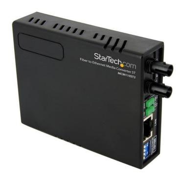
The MCM110ST2 10/100 Multi Mode ST Fiber Ethernet Media Converter (2 km) creates a cost-effective Ethernet to fiber link, transparently converting to/from 10Base-T or 100Base-Tx Ethernet signals and 100Base-Fx optical signals to extend an Ethernet network connection over a multimode fiber backbone.
