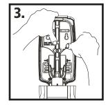
Press firmly on back plate for 30 seconds.
