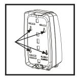
This dispenser is equipped with a universal back plate to allow for easy installation. Before drilling, open dispenser and check existing hard-ware on wall for alignment.
