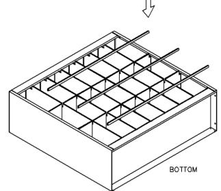
10. The grooves in the front of each plastic strip hold the paper labels provided. Separate each label along the perforations; then insert in the bottom groove, and push the label into place, tucking the top of label into the top groove with your fingernail. (Labels can be created using a PC and printer or typewriter as desired, but before separating.)
