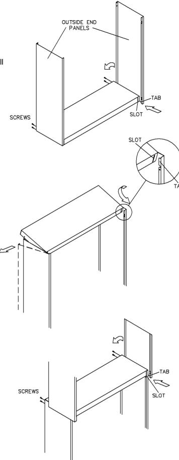
3. Install top 2" thick shelf by sliding onto tabs of outside end panels. Pull out the back edges of the outside end panels so the shelf can be lowered into place; then return outside end panels to their original position.
