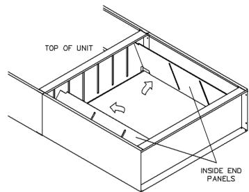
7. Install one corrugated shelf into the slots in the inside end panels, with the short folded side of the shelf on the <u>bottom</u>. Repeat with the remaining shelves in both upper and lower levels, ending with the last shelf in each level resting on the bottom of that level.
