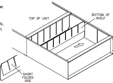
8. Place a corrugated insert ( with notch at the bottom front) into a corrugated divider. Fold small flaps at bottom of divider outwards. Now install corrugated divider, making sure the folded flaps fit <u>under</u> bottom shelf in each level, and top of divider fits into slots in header panel. Finally, press divider down firmly until flush with shelves. Repeat with remaining five dividers and inserts in upper level; then install 6 dividers and inserts in lower level.
