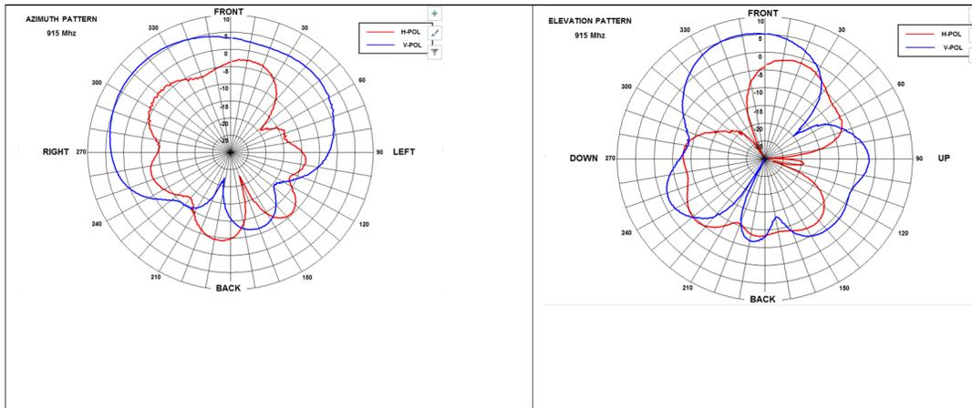
If the end product is typically installed against a wall, only the front facing radiation will be evaluated. If the end product is typically mounted on a pole, only the bottom hemisphere will be evaluated.
