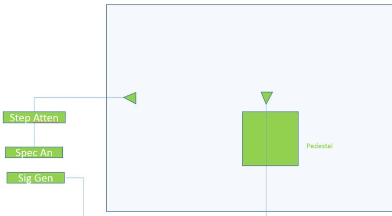
Now change the configuration to prepare for the actual test. First measure the conducted power out of the loTR's external antenna port. The loTR shall be placed inside of a shielded enclosure (e.g. Ramsey shield box).
