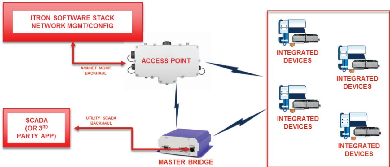
This figure shows how NIC-embedded devices communicate in a typical utility environment.
