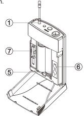
With the transmitter turned off, insert two standard AA(1.5V) batteries, making sure that the positive and negative polarity markings are oriented correctly. Although NI-CAD rechargeable batteries can be used, this transmitter cannot be recharged. Warning: do not insert the battery upside down or it may cause serious damage to your transmitter and will void the warranty.
