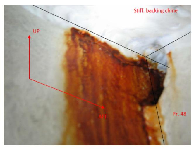
A 4-inch crack in the hull was allowing water in and led to significant rusting. The Navy's Crack Monitoring team did not know how long the crack existed before being discovered.
