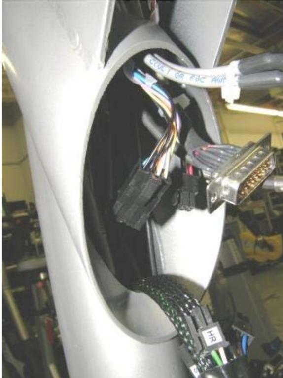
6.4 Connect the HR, shifter/trigger, steering cables from the console to the matching handlebar. Finally, connect the large 26 pin D-Sub connectors together. Ensure that all cabling is positioned properly for the plastics to go back on.
