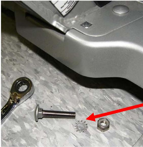
**Reinstall using new star washer**
