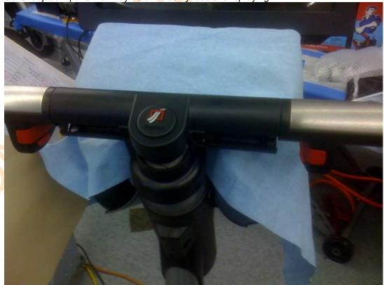
4.1.4. Remove plastic center cover and inspect the part for damages. If the part shows signs of damage, especially at the threaded insert which could affect re-assembly, a replacement part can be ordered under part number 8300.0210.01
