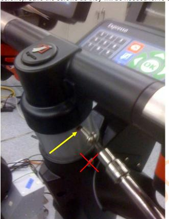
4.1.2. Remove the 4 screw holding the lower center plastic cover in place. Save the screws as they will be needed for re-assembly:
