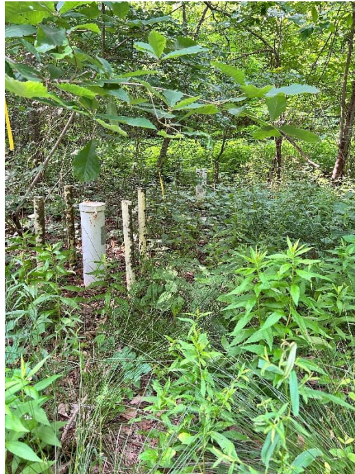
Photograph 11. Typical above ground well completion in wooded area.
