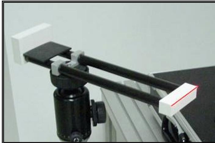
Figure 19 – Artefact correct position. Correct laser line position on the front plane.
