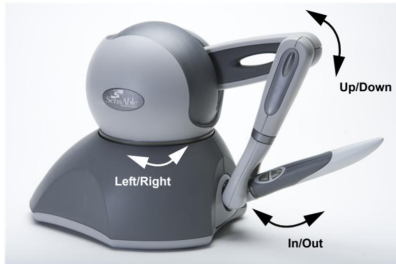
**Macro movements. Showing movement of the Phantom Omni arm and the body.**
