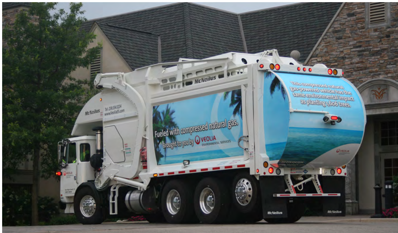
McNeilus is a leader in the CNG refuse truck market with several different platforms and vehicles using CNG fuel.
