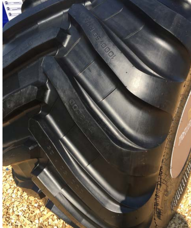
Trelleborg's TM3000 is a VF tire standardized for spreader and sprayer applications with a D rated load index for road speeds of up to 40 mph.
