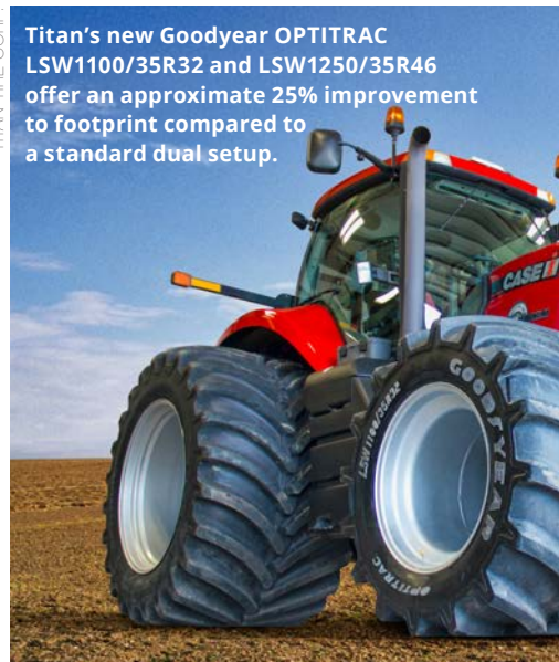
New Holland Agriculture is now offering Titan LSW tires on its T8 tractor line direct from the factory due to the reduced soil compaction benefits they offer.
