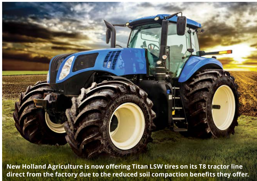
Titan's new Goodyear OPTITRAC LSW1100/35R32 and LSW1250/35R46 offer an approximate 25% improvement to footprint compared to a standard dual setup.
