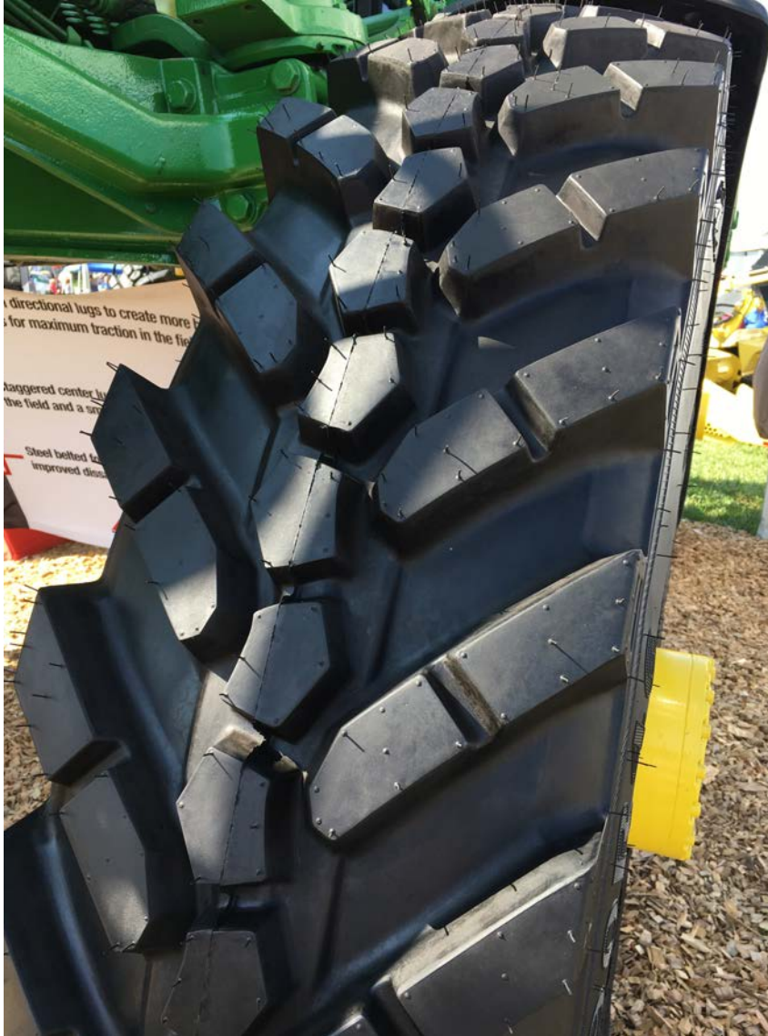
ABOVE: To mitigate heat buildup, the Agriflex 363 features a large tread face to distribute heat over a larger area, as well as more rubber in the contact patch to dissipate heat.
