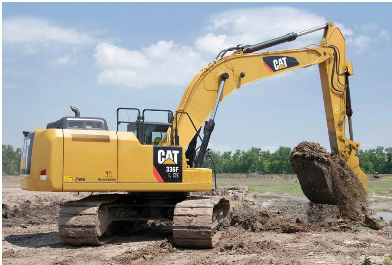
The Caterpillar 336F XE hydraulic hybrid excavator burns up to 25% less fuel than the standard 336F model while delivering the same level of production.
