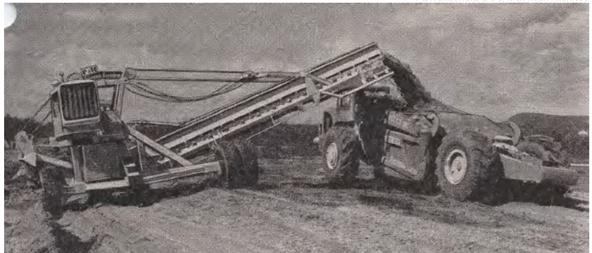
The closest competitor to a BV was the Sierra Loader, developed by C&D Manufacturing and acquired by P&H. Note the extra-wide gauge rear axle and the much wider working width compared to a BV. This one is loading what appears to be a Heil or early International Harvester motor scraper; ironically, advances in scraper design and size were the driving force in the obsolescence of BVs and Sierra Loaders.
