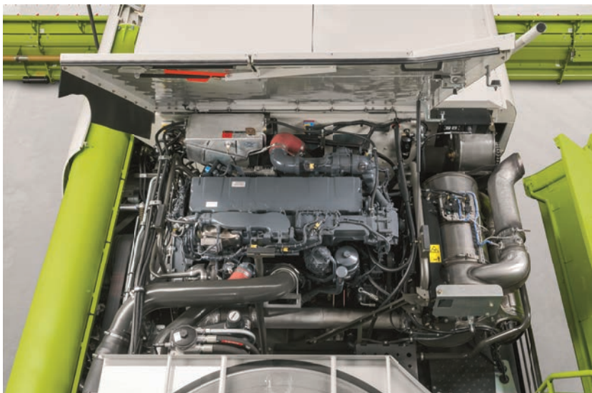
DYNAMIC COOLING pushes fresh, cool air into the engine compartment to prevent overheating.
