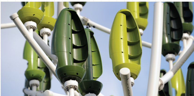
The “leaves” of Wind Trees are miniature turbines. They can move in light breezes.
