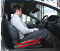
2. Move the seat forward until one can easily and fully depress the brake and accelerator.
