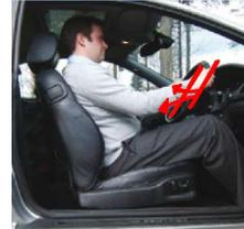
7. Adjust the head rest with the top of the rest between the top of the ears and top of the head. Headrest should be less than 2 inches from the back of the head.
