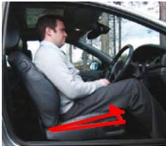
4. Adjust back rest so it provides continuous support along the length of the back and is in contact up to shoulder height.
