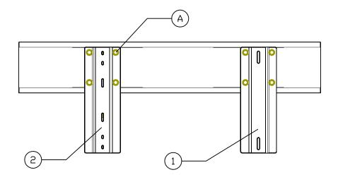
HORIZONTAL MOUNTING BRACKETS (1,2) MUST BE PARALLEL WITH FRAME RAIL
