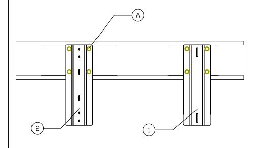
USE ALL PROVIDED GRADE 8 FASTENERS AND MANUFACTURED HOLES
