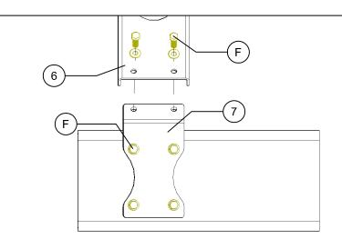
USE ALL PROVIDED GRADE 8 FASTENERS AND MANUFACTURED HOLES
