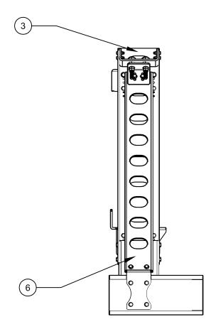
CROSS BAR(6) MUST BE PLACED PARALLEL TO VERTICAL STANCHION(3)
