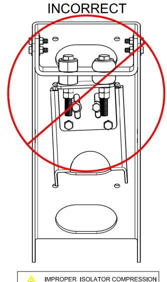
IMPROPER ISOLATOR COMPRESSION CAN LEAD TO ISOLATOR AND BRACKET FAILURE
