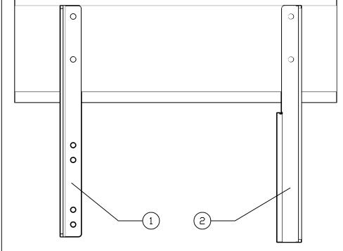
OUTSIDE FRAME BRACKET (1) AND INLET MOUNTING ANGLE (2) MUST BE PARALLEL WITH ONE ANOTHER AND PERPENDICULAR TO FRAME RAIL
