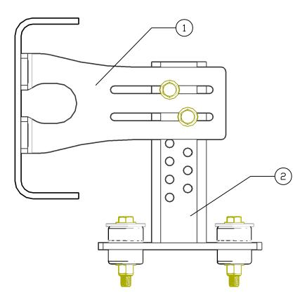
INSIDE FRAME BRACKET (1) AND ADJUSTABLE T BRACKET (2) MUST BE PERPENDICULAR WITH ONE ANOTHER AND PARALLEL TO FRAME RAIL
