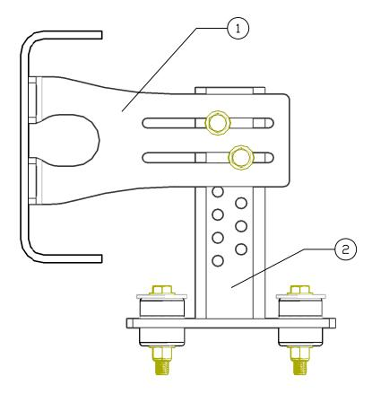
INSIDE FRAME BRACKET (1) MUST SEAT FLUSH
