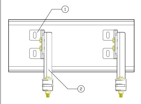
INSIDE FRAME BRACKET (1) AND ADJUSTABLE T BRACKET (2) MUST BE PERPENDICULAR WITH ONE ANOTHER AND PARALLEL TO FRAME RAIL
