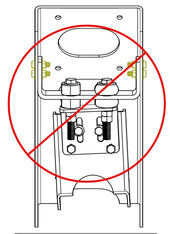
IMPROPER ISOLATOR COMPRESSION CAN LEAD TO ISOLATOR AND BRACKET FAILURE
