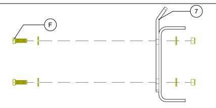
LOWER CROSS BAR BRACKET (7) MUST SEAT FLUSH TO FRAME RAIL
