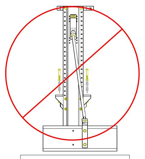
FAILURE TO INSTALL CROSS BAR (2) PARALLEL TO VERTICAL STANCHION (4) CAN COMPROMISE BRACKET INTEGRITY AND RESULT IN BRACKET FAILURE AND OR DAMAGE TO FILTER
