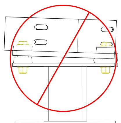
IMPROPER ISOLATOR COMPRESSION BETWEEN UPPER CAB MOUNT (1) AND FILTER MOUNT CHANNEL (2) CAN RESULT IN BRACKET FAILURE AND OR DAMAGE TO FILTER
