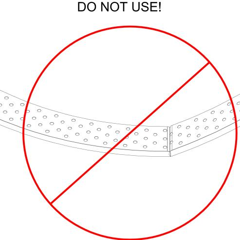
DO NOT USE GASKET THAT HAS BEEN BROKEN, BENT, OR OTHERWISE DAMAGED!
