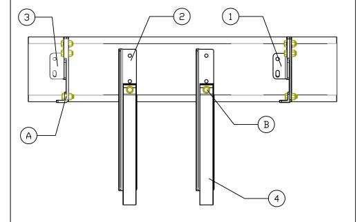
ALL BRACKET COMPONENTS OF DES M5043 MUST BE PARALLEL WITH ONE ANOTHER AND PERPENDICULAR TO FRAME RAIL
