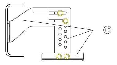
INLET AND OUTLET MOUNTING BRACKET ASSEMBLY(1,3) MUST BE PARALLEL WITH ONE ANOTHER AND PERPENDICULAR WITH FRAME RAIL
