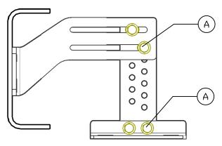
INLET AND OUTLET MOUNTING BRACKET ASSEMBLY(1,3) MUST BE PARALLEL WITH ONE ANOTHER AND PERPENDICULAR WITH FRAME RAIL
