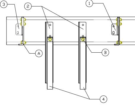
ALL BRACKET COMPONENTS OF DES M5043 MUST BE PARALLEL WITH ONE ANOTHER AND PERPENDICULAR TO FRAME RAIL
