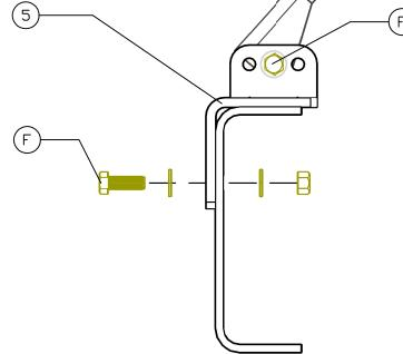
LOWER CROSS BAR BRACKET (5) MUST SEAT FLUSH TO FRAME RAIL
