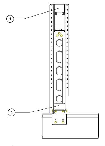
CROSS BAR(4) MUST BE PLACED PARALLEL TO 56"VERTICAL STANCHION(1)
