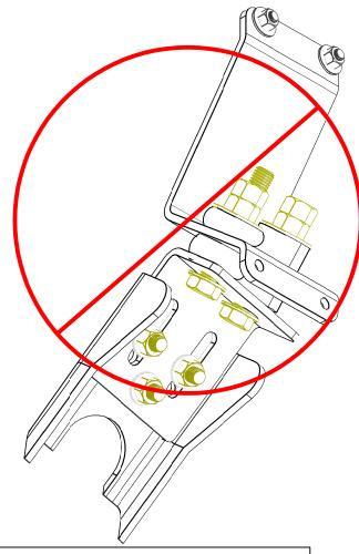
IMPROPER ISOLATOR COMPRESSION CAN LEAD TO ISOLATOR AND BRACKET FAILURE
