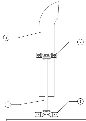
18" STABILIZER ASSEMBLY (1) MUST BE MOUNTED IN LINE WITH FILTER OUTLET HAT AND 36" CHROME EXHAUST STACK (4)
