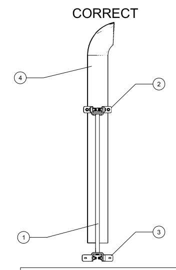
36" STABILIZER ASSEMBLY (1) MUST BE MOUNTED IN LINE WITH FILTER OUTLET HAT AND 60" CHROME EXHAUST STACK (4)
