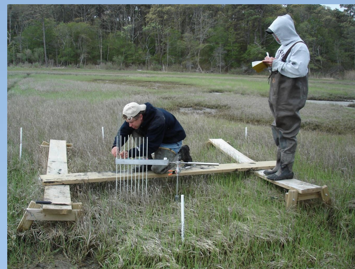
Figure 1: Taking Sediment Elevation Table (SET) measurements in Delaware's inland bays.
