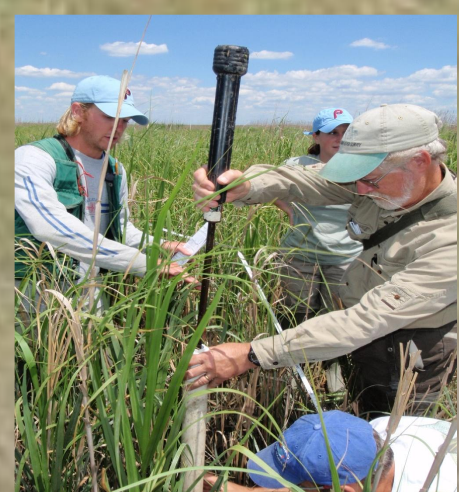
Figure 7: Measuring bearing capacity in wetlands.
