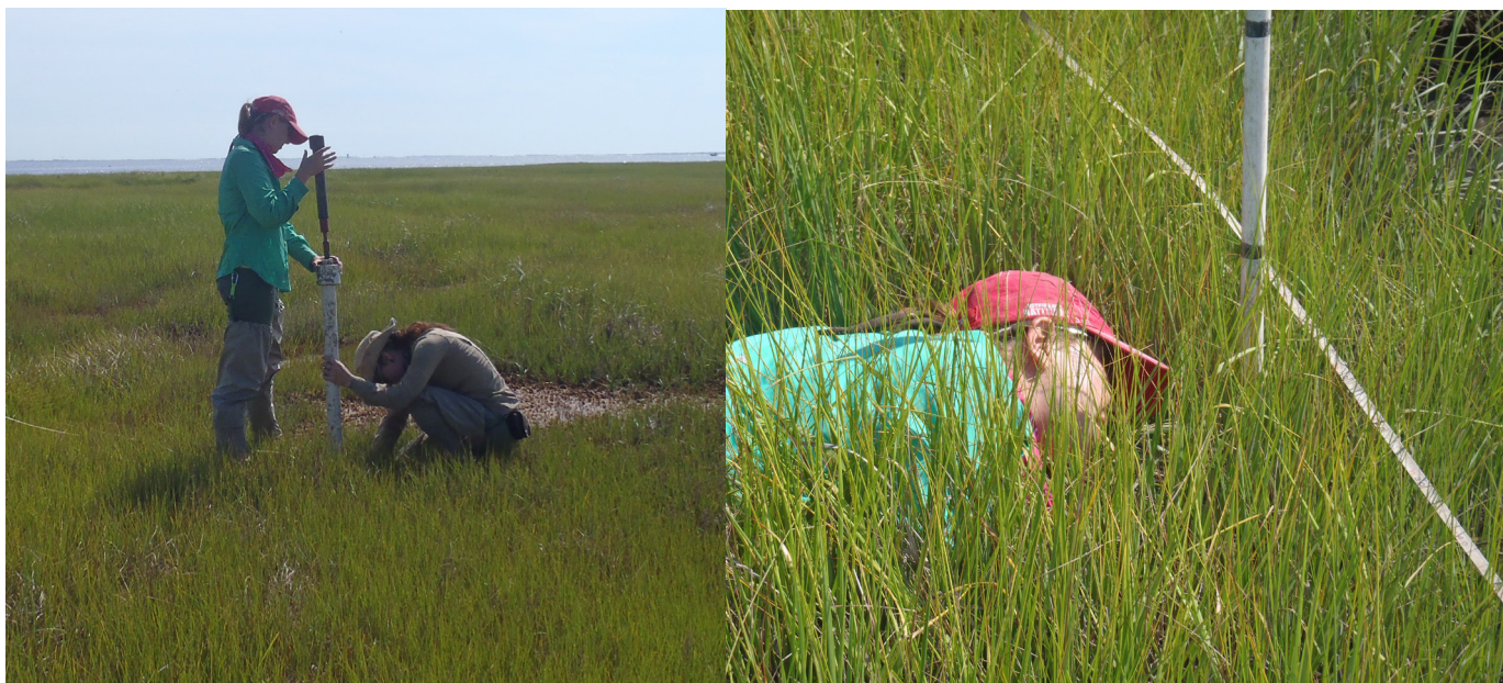
Figure 14. PDE and BBP staff using Mid-TRAM field techniques: on the left, bearing capacity; on the right, looking through Spartina alterniflora to obtain horizontal vegetation obstruction (i.e. canopy density)
