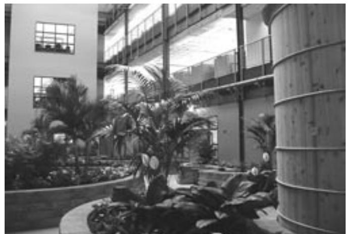
*A view of the first floor atrium and 4,000-gallon wooden cistern that collects rainwater from the rooftop at PA DEP’s new facility in Norristown, Pennsylvania.*
