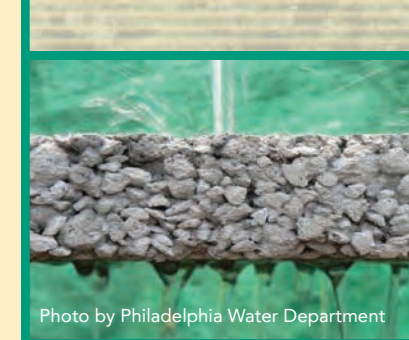
Porous pavement soaks up water
