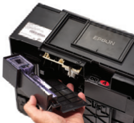
8 Slide the Ink Pad left to remove
