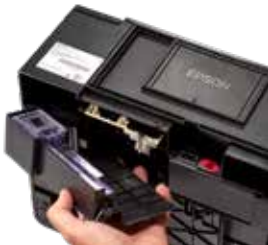
8 Slide the Ink Pad left to remove
