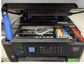
4. When the screen says, "Replace ink cartridges", lift the top of the printer.
