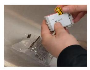
5. Remove cartridge from its packaging, then remove the yellow tab.
