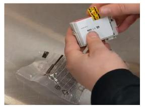
6. Remove the new cartridge from its packaging, then remove the yellow tab.
