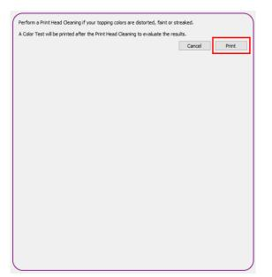
3. Insert a sheet of plain printer paper, then press the Print button.
