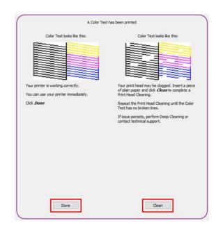
4. If the problem has cleared up, press the Done button. If there are still many gaps in the Color Test, we suggest doing a total of 4 Print Head Cleanings before moving on to the next step.
