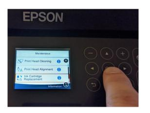
2. Press the down arrow until the "Ink Cartridge Replacement" icon, then press OK.
