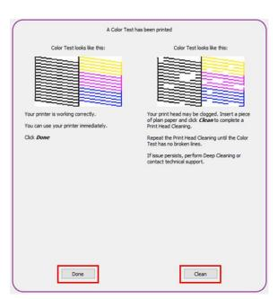
4. If the printed lines have no breaks or a few, press the Done button. If there are a significant number of breaks in the test lines, we suggest trying a Print Head Cleaning. Begin the cleaning by pressing the Clean button.
