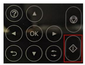
5. Press the diamond shaped button. Wait for the print head to stop moving.
