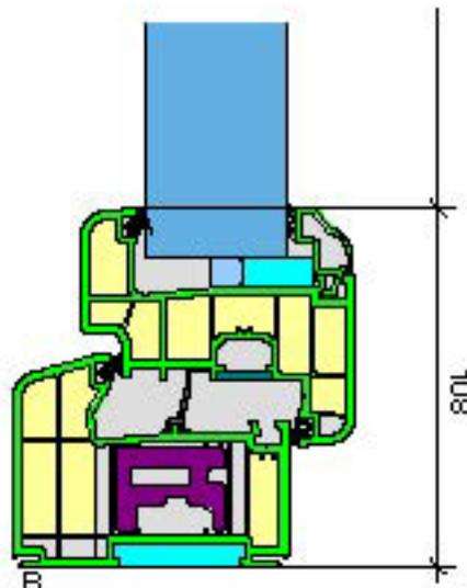
Pictured is a cross section of Deceuninck North America's Revolution XL™ Tilt & Turn Passive House Edition window, which has earned certification as a Passive House Component.
