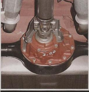
The "3.00" written in white refers to final-drive ratio. The four-speed KR was normally delivered with a 3.50:1 rear axle ratio. Points would be deducted if the owner did not have good documentation with the car to back up the variation on the axle marking from the accepted standard.
