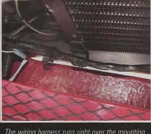
The wiring harness runs right over the mounting bracket for the A/C condenser on all big-block A/C Mustangs and Shelbys. The black plastic bracket cover that protects the harness from chafing against the raw steel is seldom found on original cars and reproductions aren't available, yet. So, what do you do? If you are restoring to concours quality, you search high and low for a surviving sample and spend \$1,500 having a dozen or so sets of them recreated.
