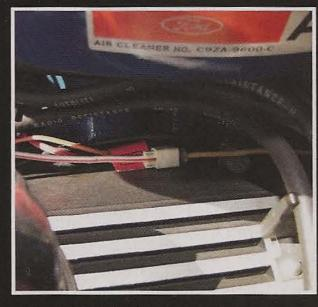
Some things that don't look original may very well be. The white scotch-lock splice into the wiring harness was a modification made during the transformation from Mustang to Shelby to tie into the up-fitted Stewart-Warner oil-pressure sensor.
