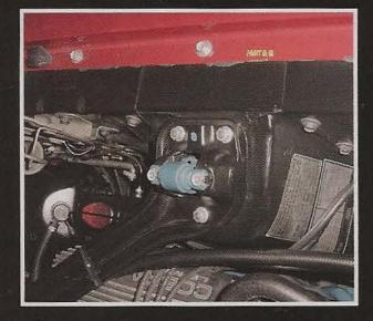
Some concours corrections are very simple. The plug wires on the left-side bank fire sequentially and must not run parallel. For better performance and more points left on the judging sheet, switch wire 5 and 7 so they cross over one another. This fix is both easy and free.
