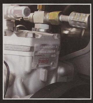
A sharp eye will also notice the reproduction A/C hose near the top of the photo, acting as a placeholder until fresh high-pressure hoses are rebuilt using original fittings.
