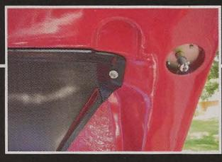
The air chamber on the fiberglass hood was originally mounted using an orange/red RTV compound no longer produced. The bead of a similar substance was used here. The sloppy, oozing effect is a correct detail. In the upper right-hand corner there is a special rivet used to fasten the chamber at the front corner, and also requires its own tool to install. One can easily spend hundreds of dollars to recreate a factory-delivered detail like this.
