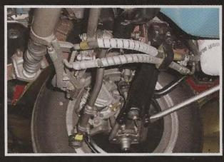
Division II cars are allowed to have their suspension components painted to prevent corrosion. Division I cars are not allowed to-bare metal remains bare metal. If this were a Division I style restoration you would see more contrast between the light shade steering adjuster sleeve and the darker hardened steel of the bands on the steering link. The same can be said for cast-iron brake caliper and heattreated spindle.
