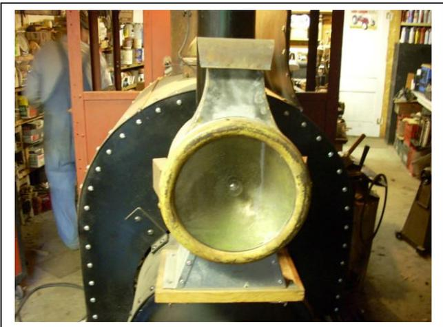
The headlamp was fashioned from a chicken water pan and a Model T headlamp mounted on the "smokebox". The riveted structure replicated the water tank around the "boiler".
