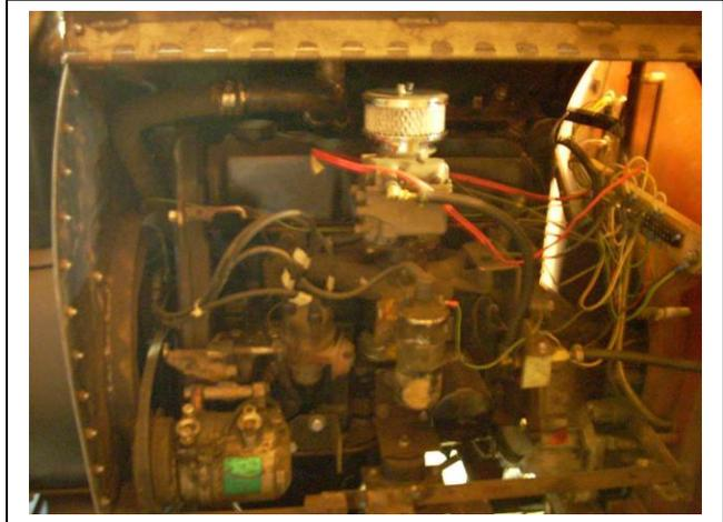
Instead of water in the tank and steam in the "boiler" Fred has inserted a Ford Ranger four-speed gasoline powered four-cylinder engine that exhausts through the stack.
