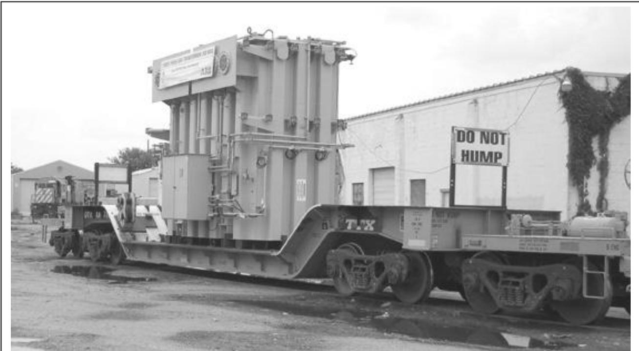
The eight-axel car, QTTX130711, carrying a Brazilian transformer to be installed in the new Tontitown SWEPCO generating plant. The car is near its load capacity of 468,000 pounds.
