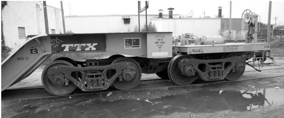
A Close-up view of the dual articulated truck assemblies on one end of the car.
