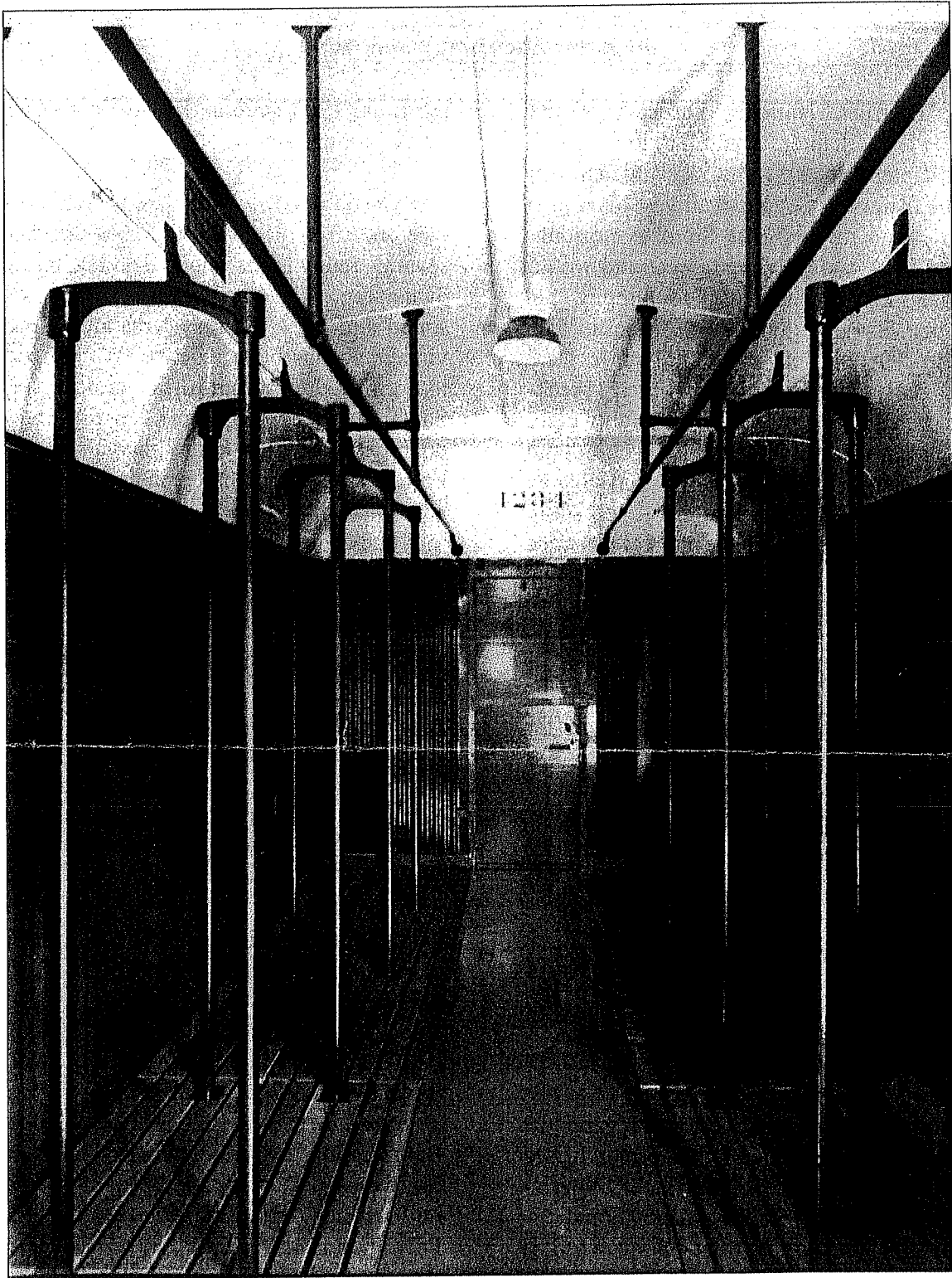
The car has two identical 19-foot compartments, one at each end, that were used to carry express items such as iced fruit and vegetables. The floor beneath the wood slats is made of tin and has drainage holes. The Chapter plans to construct an exhibit on the Railroad History of Northwest Arkansas in one compartment. (From the Barriger Collection of the Mercantile Library of St. Louis at the University of Missouri, St Louis)
