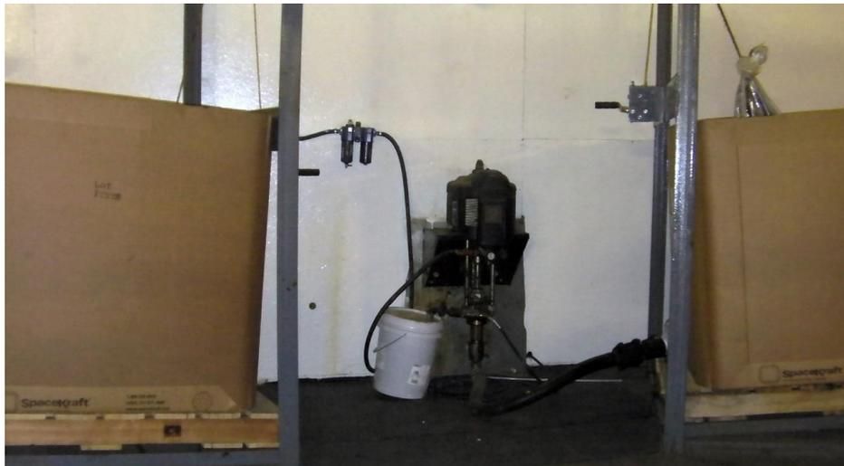
**CAPTION:** Previously, the undercoating had been delivered in 55-gallon drums, resulting in downtime when they emptied. The modified Tectyl undercoating allowed the product to be delivered through a 330-gallon tote system – when one tote is empty, the valve is closed and the second tote valve is opened. No interruptions to production.
