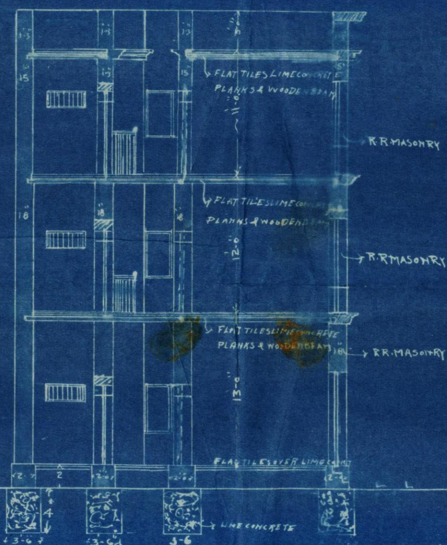
SECTION ON LINE A-B
