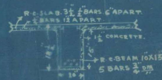
SECTION ON C.D. SCALE 1/2" = 1' FOOT.
