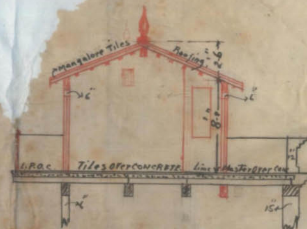
Section On line A-B.
