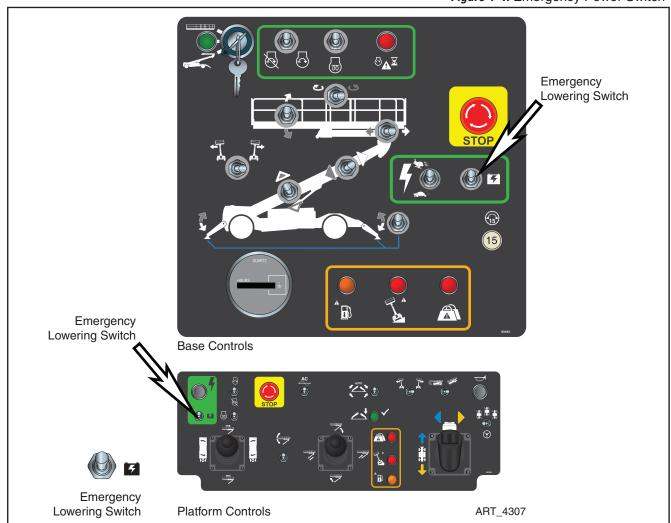
Figure 1-4: Emergency Power Switch
