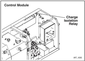
Figure 2-15: Generator Relay
