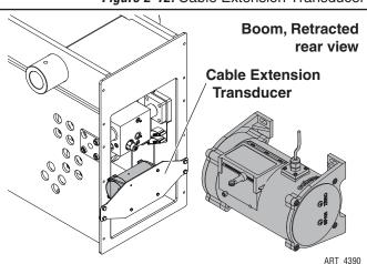
Figure 2-12: Cable Extension Transducer
