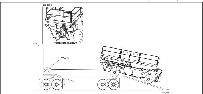
Figure 1-6: Loading the Machine
