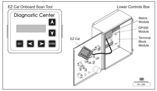
Figure 2-26: GP440 Module & VCCM Locations
