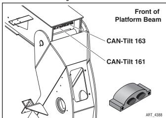
Figure 2-6: Platform Beam CAN-Tilts
