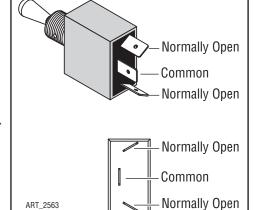
Figure 2-19: Toggle Switch, 1-Pole 2-Position
