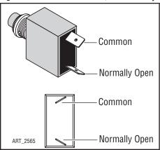
Figure 2-23: Emergency Stop Switch
