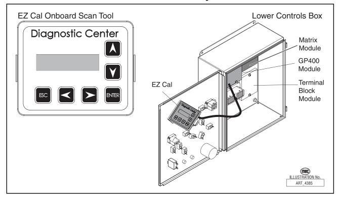
Figure 2-26: GP440 Module & VCCM Locations
