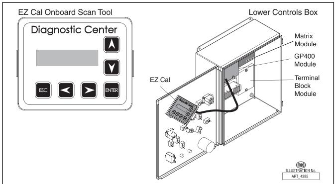
Figure 4-5: Onboard EZ-Cal Scan Tool & GP400 Module
