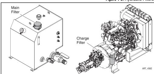
Figure 1-2: Hydraulic Filters
