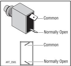
Figure 2-23: Emergency Stop Switch
