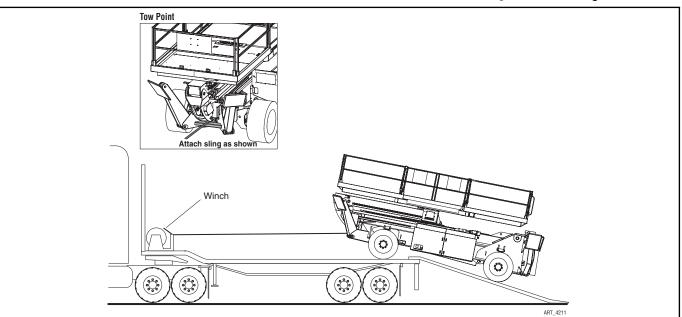
Figure 1-6: Loading the Machine
