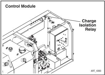
Figure 2-15: Generator Relay
