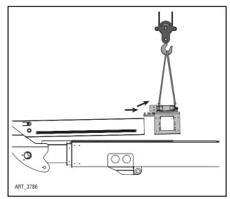
UNIT CONTAINS THE BRAKE, WHICH PREVENTS THE CARRIAGE FROM SLIDING FREELY. REMOVING THIS UNIT WILL REMOVE THE BRAKE.
