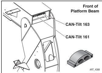
Figure 2-6: Platform Beam CAN-Tilts
