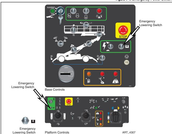
Figure 1-4: Emergency Power Switch
