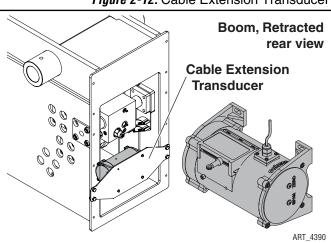
Figure 2-12: Cable Extension Transducer
